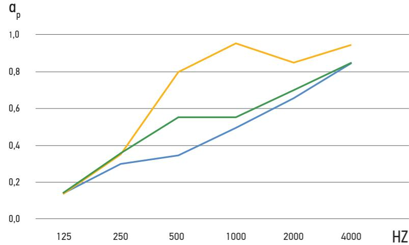
Measurement of the sound absorption of acoustic foam
