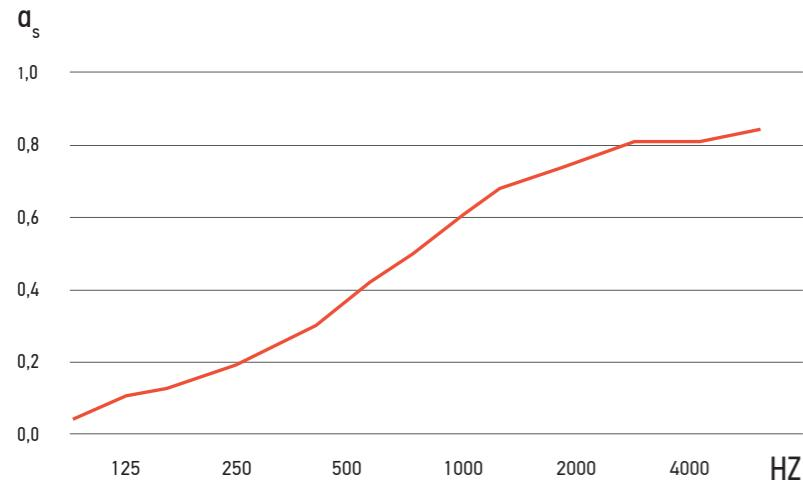
The acoustic foam used in the JAZZ Silent Box absorbs sound effectively, is fire-resistant (DIN 4102 (B1), EN13501, UNI 9177 (Class 1)).
